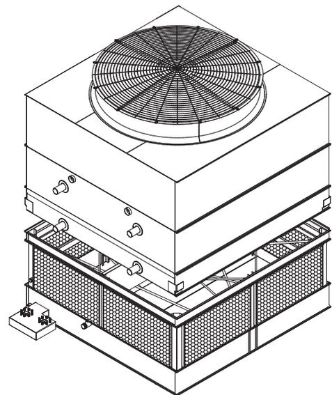
Figure 8 - Mating Upper Section to Basin Section
