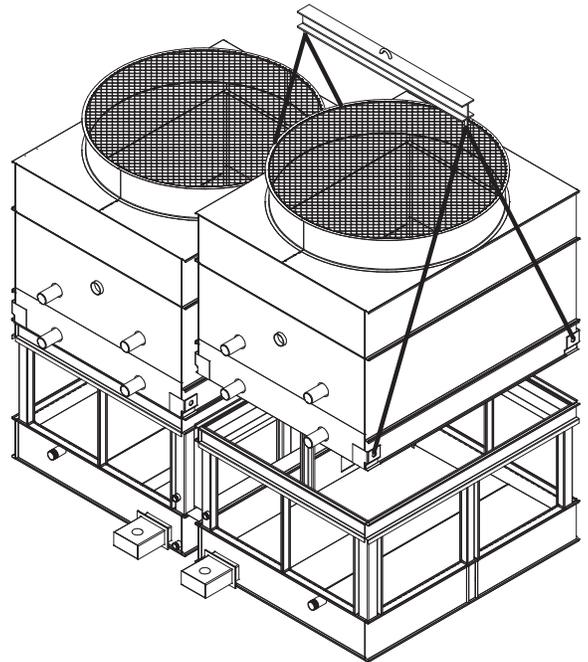
Figure 16 - Mating Fan/Coil Section to Basin Section
