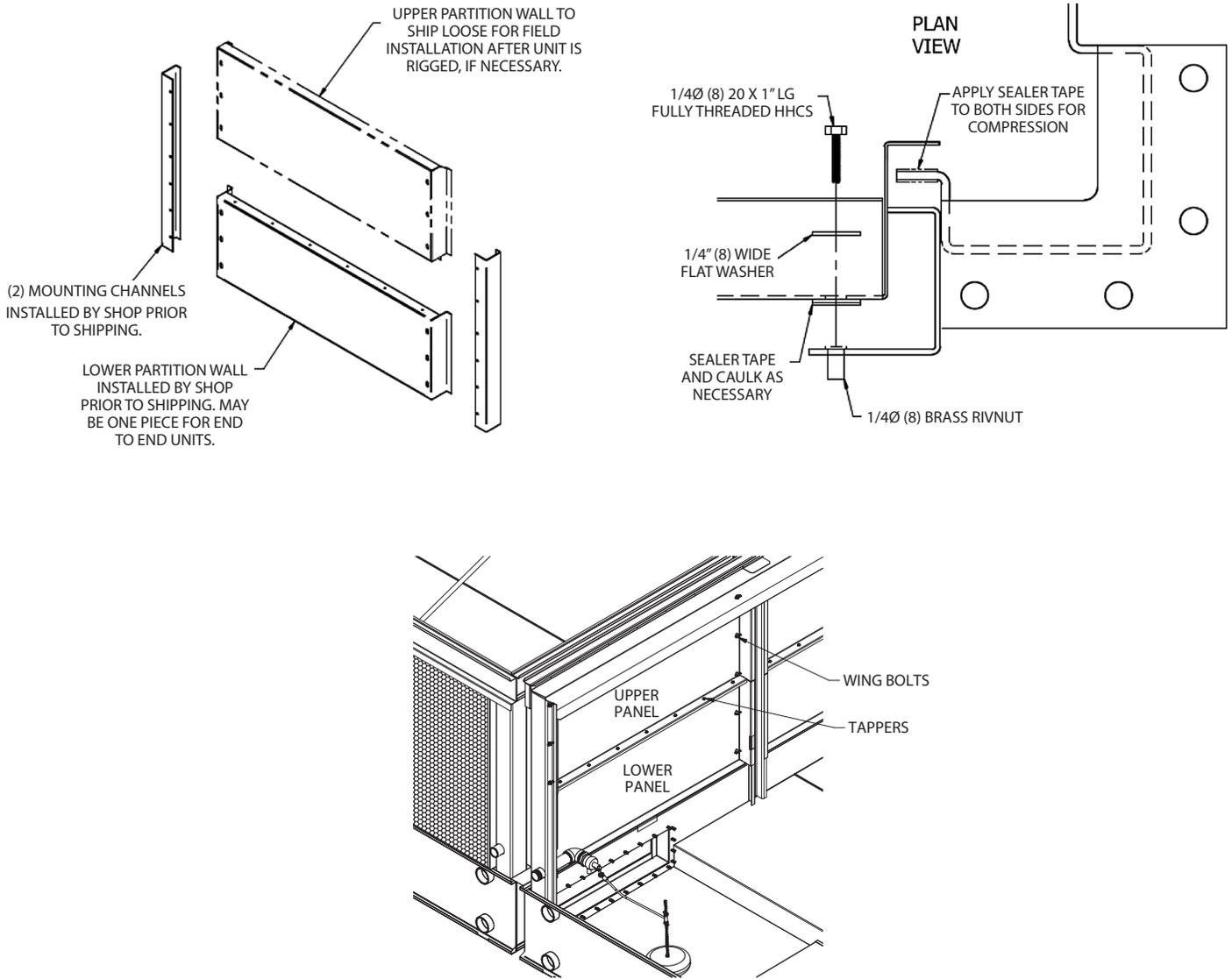
Figure 17 - Upper Partition/Firewall Installation in Field
