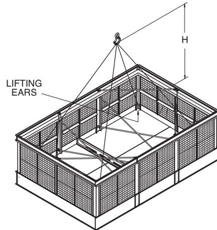
**Figure 1a** - Basin Section up to 21' (6.4m) long
