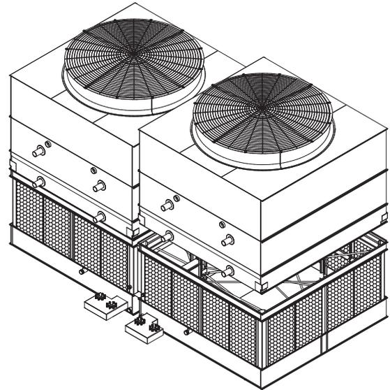
Figure 9 - Mating Upper Section to Basin Section
