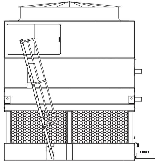
**Figure 25b** - Side View of Ladder Assembly
