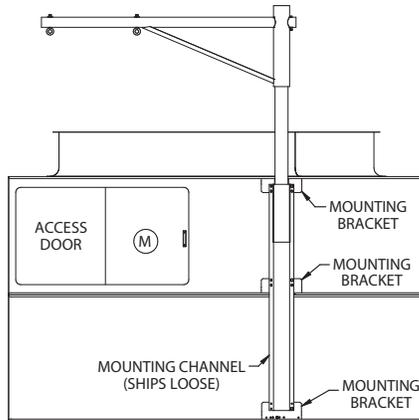
Figure 20 - Dual-Point Davit Arrangement
