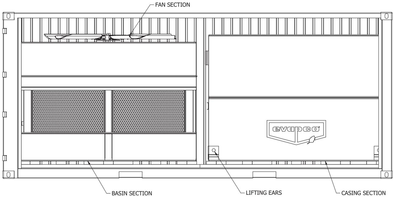
Figure 12 - 20' Standard Height Container Shipment
