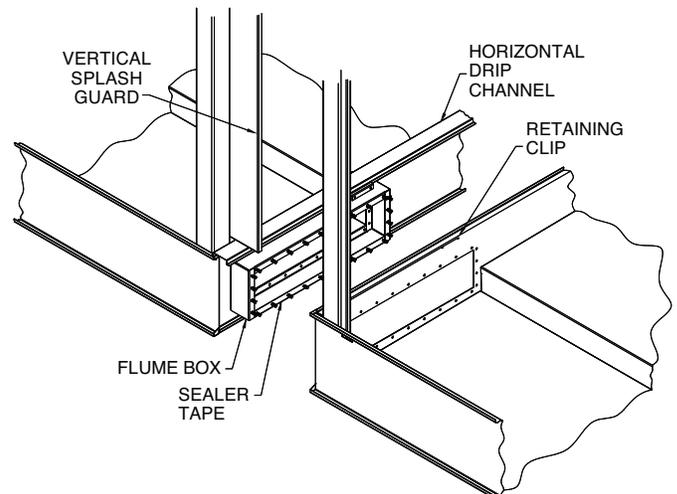
**Figure 2** - Equalizer Flume Connection, 12' (3.6m) Wide Models
