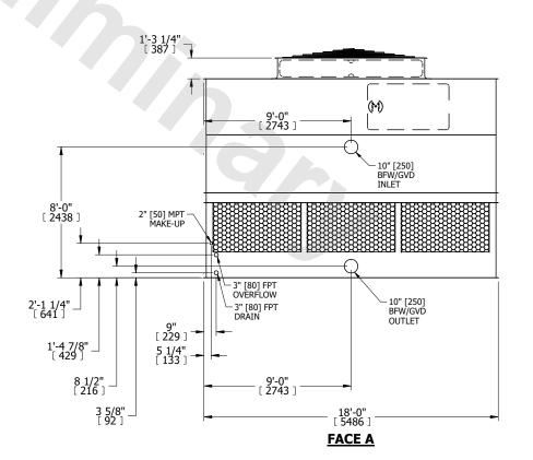
DRAWN BY: KDS NO. OF SHIPPING SECTIONS **SHIPPING** OPERATING HEAVIEST SECTION 9360 lbs+ [4250] kg+ 16960 lbs+ [7695] kg+ 5810 lbs+ [2640] kg+ WEIGHT WEIGHT WEIGHT
