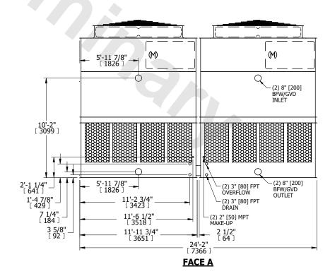
SHIPPING WEIGHT 16560 lbs+ [7515] kg+ OPERATING WEIGHT 28980 lbs+ [13150] kg+ HEAVIEST SECTION WEIGHT 5740 lbs+ [2605] kg+ NO. OF SHIPPING SECTIONS 4 DRAWN BY: KDS
