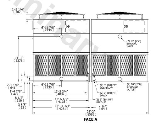
SHIPPING WEIGHT 19180 lbs+ [8700] kg+ OPERATING WEIGHT 33840 lbs+ [15350] kg+ HEAVIEST SECTION WEIGHT 6540 lbs+ [2970] kg+ NO. OF SHIPPING SECTIONS 4 DRAWN BY: KDS
