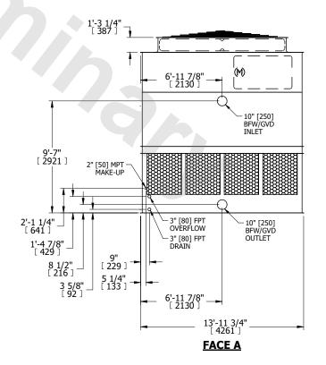
DRAWN BY: KDS NO. OF SHIPPING SECTIONS **SHIPPING** OPERATING HEAVIEST SECTION 9410 lbs+ [4270] kg+ 6540 lbs+ [2970] kg+ 16740 lbs+ [7595] kg+ WEIGHT WEIGHT WEIGHT
