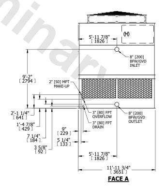
SHIPPING WEIGHT 8140 lbs+ [3695] kg+ OPERATING WEIGHT 14350 lbs+ [6510] kg+ HEAVIEST SECTION WEIGHT 5740 lbs+ [2605] kg+ NO. OF SHIPPING SECTIONS 2 DRAWN BY: KDS
