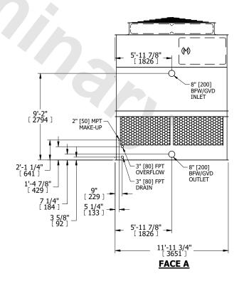
SHIPPING WEIGHT 8040 lbs+ [3650] kg+ OPERATING WEIGHT 14250 lbs+ [6465] kg+ HEAVIEST SECTION WEIGHT 5640 lbs+ [2560] kg+ NO. OF SHIPPING SECTIONS 2 DRAWN BY: KDS
