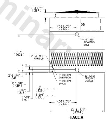
DRAWN BY: KDS NO. OF SHIPPING SECTIONS **SHIPPING** OPERATING HEAVIEST SECTION 9020 lbs+ [4095] kg+ 6150 lbs+ [2790] kg+ 16350 lbs+ [7420] kg+ WEIGHT WEIGHT WEIGHT
