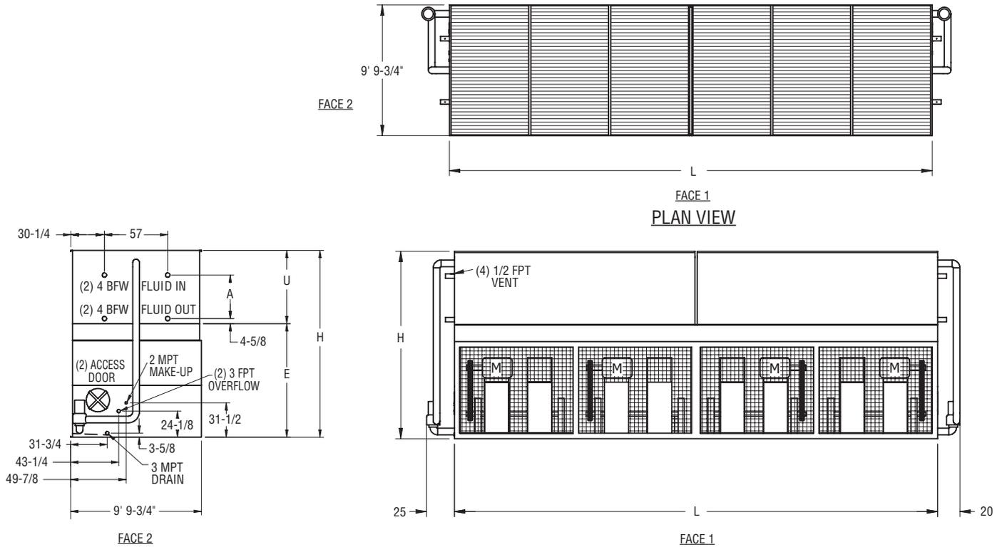
Note: The number of coil connections doubles when the flow rate exceeds 1800 gpm on 10x36 models. This required option is referred to as the High Flow coil configuration.
