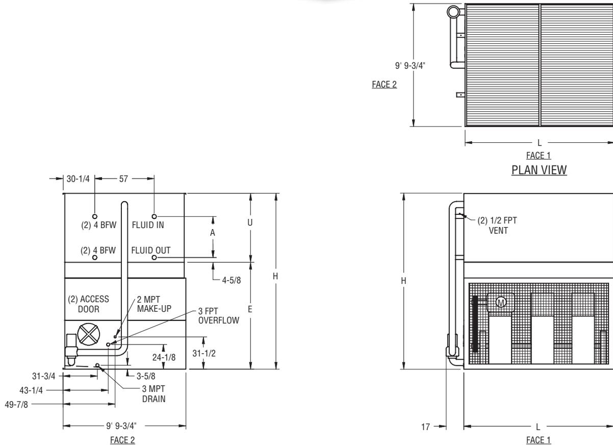
Note: The number of coil connections doubles when the flow rate exceeds 900 gpm on 10x12 models. This required option is referred to as the High Flow coil configuration.
