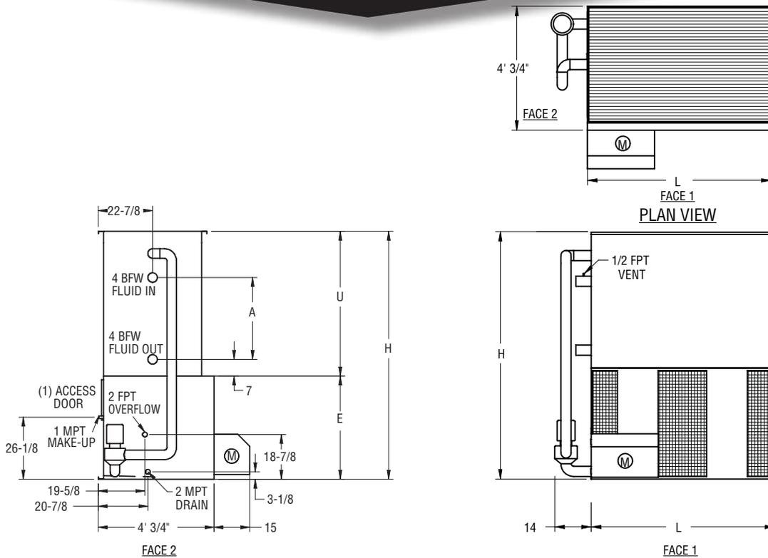
Note: The number of coil connections doubles when the flow rate exceeds 450 gpm on 4x6 and 4x9 models. This required option is referred to as the High Flow coil configuration.
