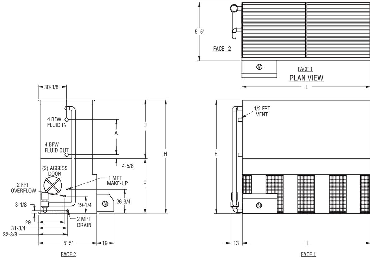
Note: The number of coil connections doubles when the flow rate exceeds 450 gpm on 5x12 models. This required option is referred to as the High Flow coil configuration.
