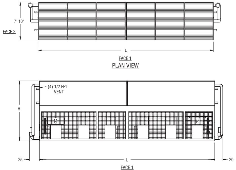
Note: The number of coil connections doubles when the flow rate exceeds 1800 gpm on 8Px36 models. This required option is referred to as the High Flow coil configuration.
