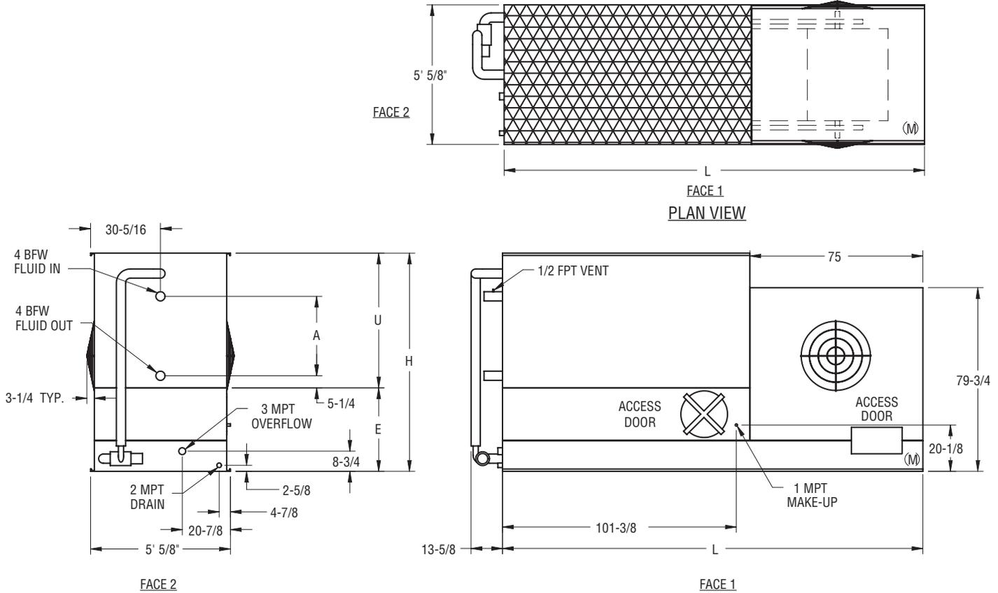
Note: The number of coil connections doubles when the flow rate exceeds 450 gpm on 5x9 models. This required option is referred to as the High Flow coil configuration.
