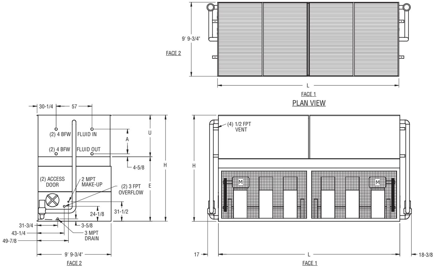
Note: The number of coil connections doubles when the flow rate exceeds 1800 gpm on 10x24 models. This required option is referred to as the High Flow coil configuration.
