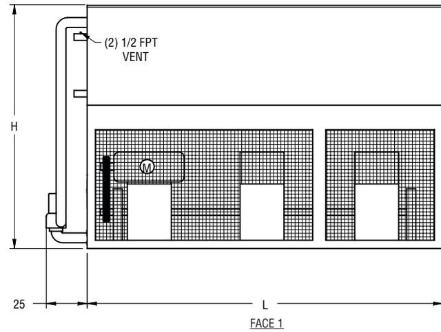
Note: The number of coil connections doubles when the flow rate exceeds 900 gpm on 8Px18 models. This required option is referred to as the High Flow coil configuration.
