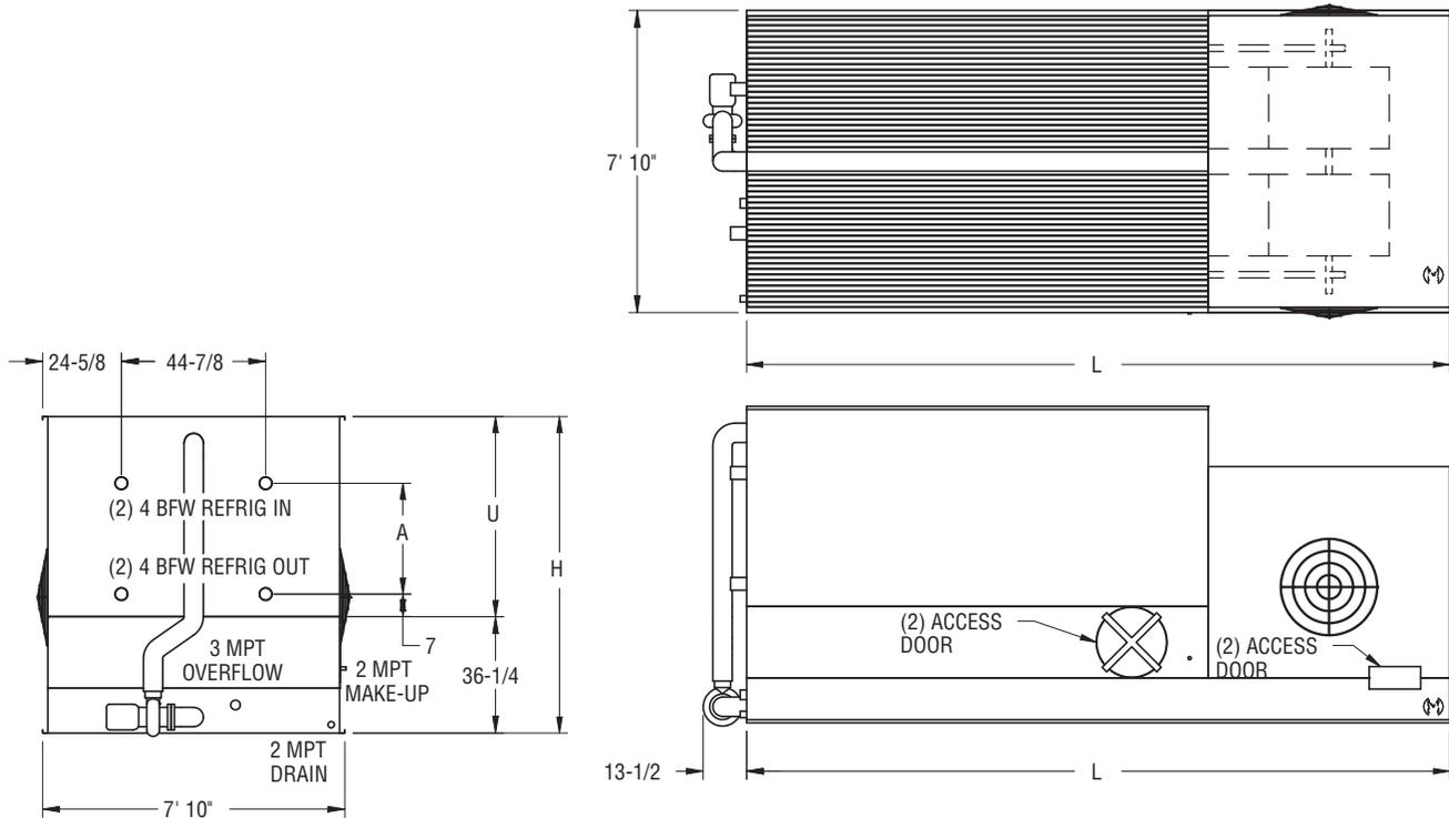
Note: The number of coil connections doubles when the flow rate exceeds 900 gpm on 8x9 and 8x12 models. This required option is referred to as the High Flow coil configuration.
