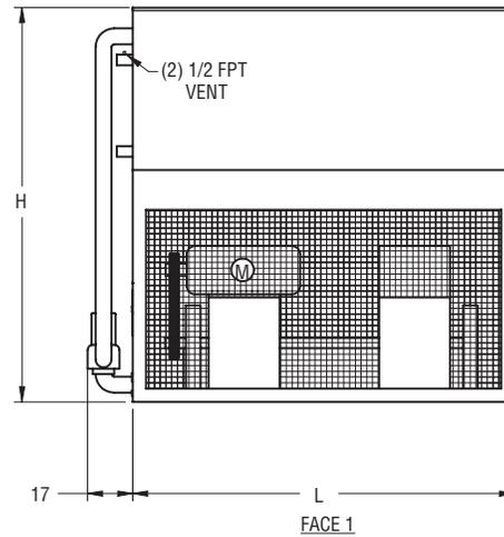
Note: The number of coil connections doubles when the flow rate exceeds 900 gpm on 8Px12 models. This required option is referred to as the High Flow coil configuration.
