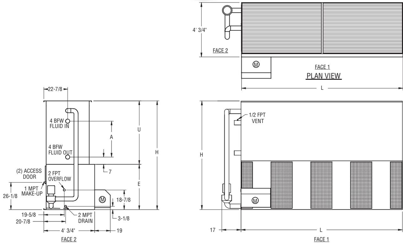
Note: The number of coil connections doubles when the flow rate exceeds 450 gpm on 4x6 and 4x9 models. This required option is referred to as the High Flow coil configuration.
