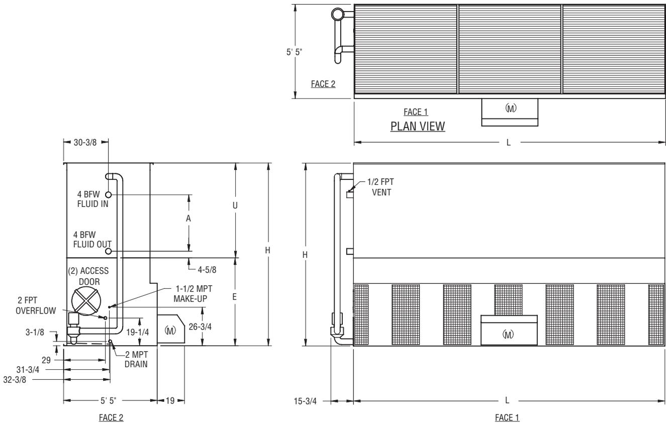
Note: The number of coil connections doubles when the flow rate exceeds 450 gpm on 5x18 models. This required option is referred to as the High Flow coil configuration.
