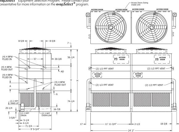
Note: The below table lists base unit dimensions and weights. See the table at the bottom Right of the Page for dry coil section dimensions and weight adds. Note: The number of coil connections doubles when the flow rate exceeds 1,800 GPM on eco-ATWB-H 10x24 models. This required option is referred to as the High Flow coil configuration.
