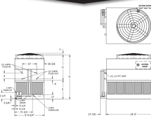
Note: The number of coil connections doubles when the flow rate exceeds 900 GPM on eco-ATWE 10x18 models. This required option is referred to as the High Flow coil configuration.
