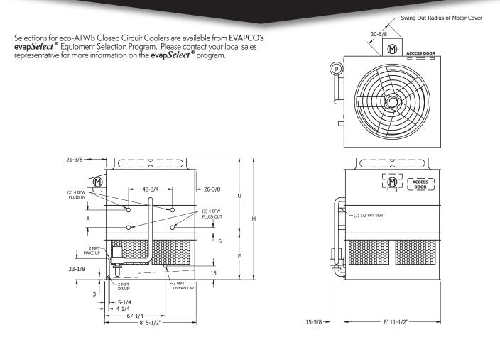
Note: The number of coil connections doubles when the flow rate exceeds 900 GPM on eco-ATW 9x9 models. This required option is referred to as the High Flow coil configuration.
