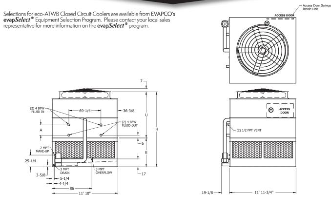
Note: The number of coil connections doubles when the flow rate exceeds 900 GPM on eco-ATW 12x12 models. This required option is referred to as the High Flow coil configuration.
