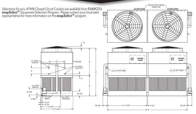
Note: The number of coil connections doubles when the flow rate exceeds 1,800 GPM on eco-ATW 10x24 models. This required option is referred to as the High Flow coil configuration.
