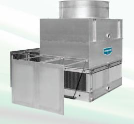
Electric immersion heaters can be added to the basin of your Advanced Technology series cooling tower. They are sized to maintain a +40° F (4.5° C) pan water temperature with the fans and system pumps off. A thermostat and low-water protection device cycle the heater on when required and prevent the heater elements from energizing unless they are completely submerged. All components are protected by rugged, weatherproof enclosures for outdoor use.
