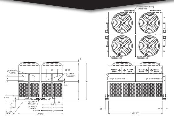
Note: The number of coil connections doubles when the flow rate exceeds 3,600 GPM on eco-ATW 20x36 models. This required option is referred to as the High Flow coil configuration.
