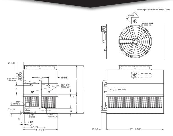
Note: The number of coil connections doubles when the flow rate exceeds 900 GPM on eco-ATW 9x14 models. This required option is referred to as the High Flow coil configuration.
