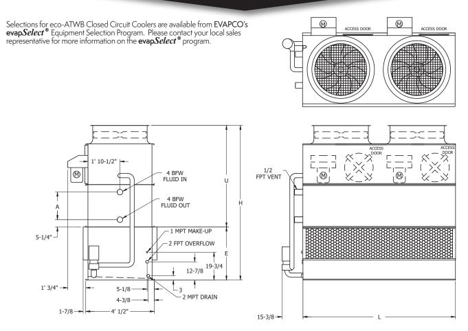
**Note:** The number of coil connections doubles when the flow rate exceeds 450 GPM on eco-ATW 4x9 and 4x12 models. This required option is referred to as the High Flow coil configuration.
