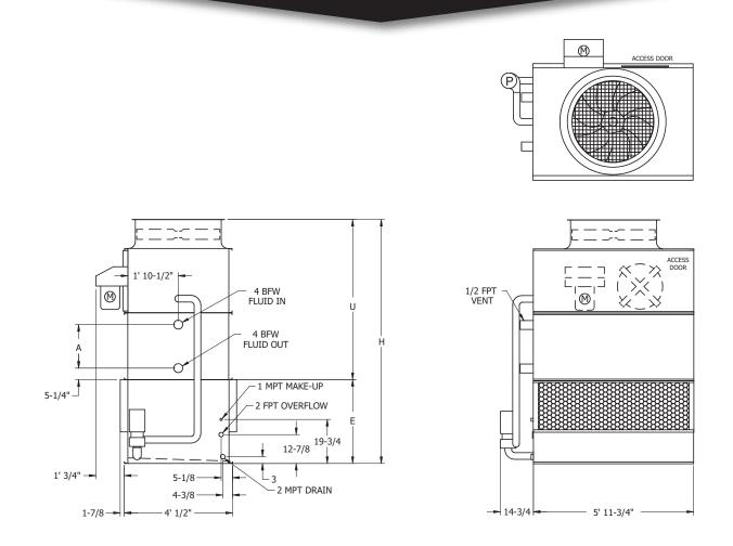
Note: The number of coil connections doubles when the flow rate exceeds 450 GPM on 4x6 models. This required option is referred to as the High Flow coil configuration.
