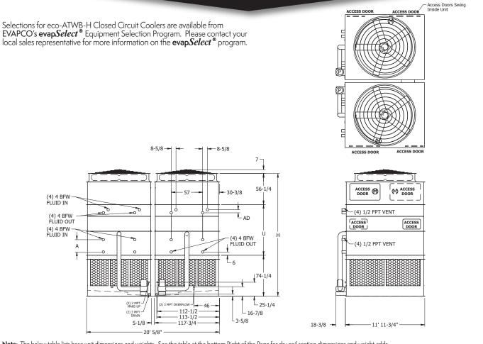
Note: The below table lists base unit dimensions and weights. See the table at the bottom Right of the Page for dry coil section dimensions and weight adds. Note: The number of coil connections doubles when the flow rate exceeds 1,800 GPM on eco-ATWB-H 20x12 models. This required option is referred to as the High Flow coil configuration.
