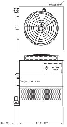
Note: The number of coil connections doubles when the flow rate exceeds 900 GPM on eco-ATW 12x14 models. This required option is referred to as the High Flow coil configuration.
