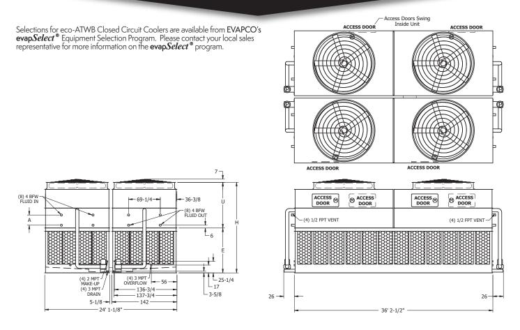
Note: The number of coil connections doubles when the flow rate exceeds 3,600 GPM on eco-ATW 24x36 models. This required option is referred to as the High Flow coil configuration.
