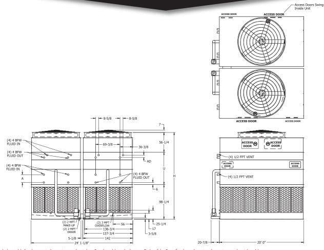
Note: The below table lists base unit dimensions and weights. See the table at the bottom Right of the Page for dry coil section dimensions and weight adds. Note: The number of coil connections doubles when the flow rate exceeds 1,800 GPM on eco-ATWB-H 24x20 models. This required option is referred to as the High Flow coil configuration.
