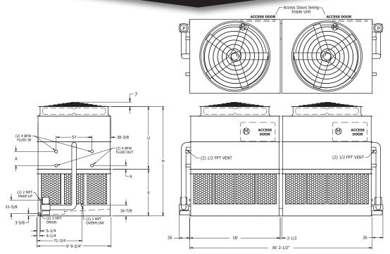
Note: The number of coil connections doubles when the flow rate exceeds 1,800 GPM on eco-ATW 10x36 models. This required option is referred to as the High Flow coil configuration.
