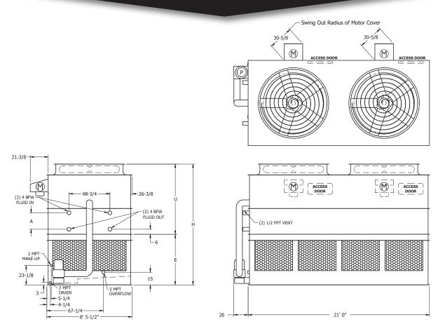
Note: The number of coil connections doubles when the flow rate exceeds 900 GPM on eco-ATW 9x21 models. This required option is referred to as the High Flow coil configuration.
