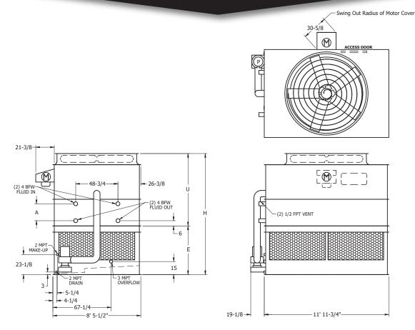
Note: The number of coil connections doubles when the flow rate exceeds 900 GPM on eco-ATW 9x11 models. This required option is referred to as the High Flow coil configuration.
