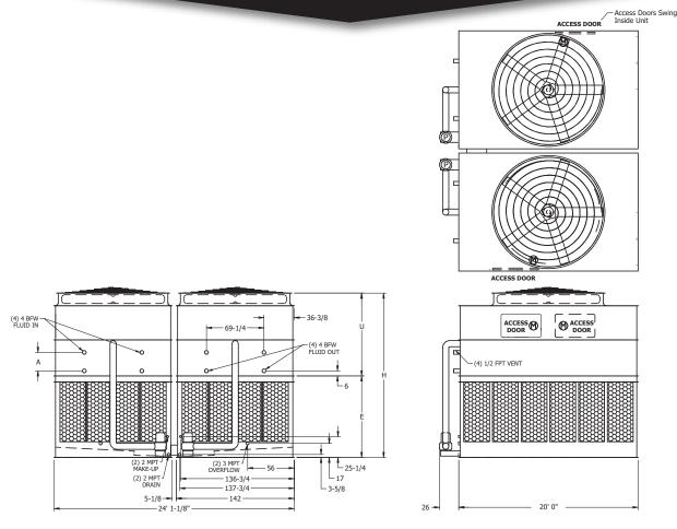
Note: The number of coil connections doubles when the flow rate exceeds 1,800 GPM on eco-ATW 24x20 models. This required option is referred to as the High Flow coil configuration.
