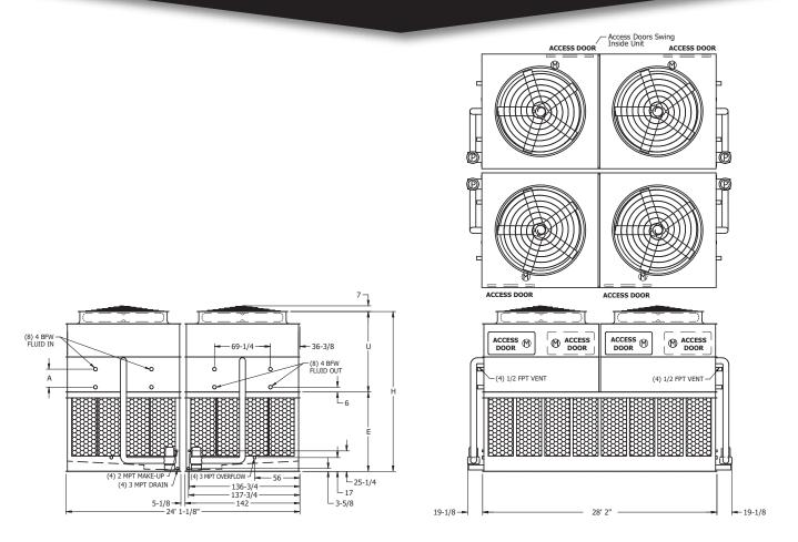
Note: The number of coil connections doubles when the flow rate exceeds 3,600 GPM on eco-ATW 24x28 models. This required option is referred to as the High Flow coil configuration.
