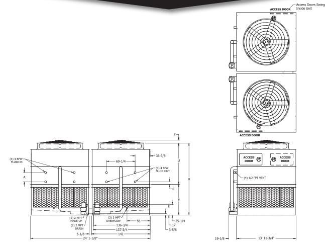
Note: The number of coil connections doubles when the flow rate exceeds 1,800 GPM on eco-ATW 24x14 models. This required option is referred to as the High Flow coil configuration.
