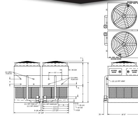
Note: The number of coil connections doubles when the flow rate exceeds 1,800 GPM on eco-ATW 20x18 models. This required option is referred to as the High Flow coil configuration.
