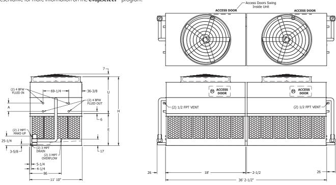
Note: The number of coil connections doubles when the flow rate exceeds 1,800 GPM on eco-ATW 12x36 models. This required option is referred to as the High Flow coil configuration.
