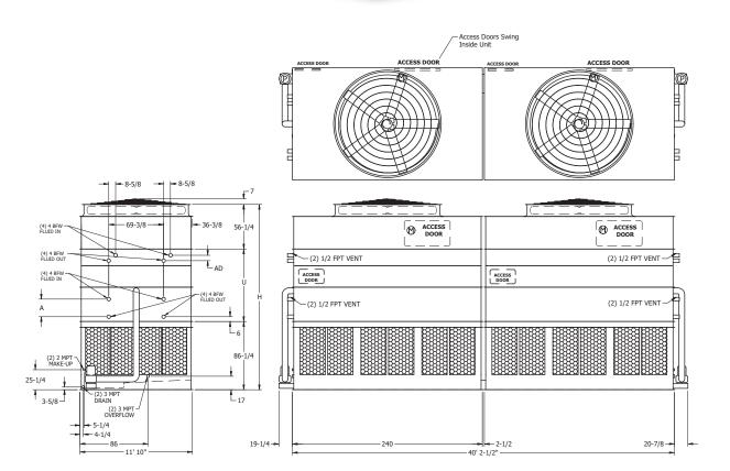
Note: The below table lists base unit dimensions and weights. See the table at the bottom Right of the Page for dry coil section dimensions and weight adds. Note: The number of coil connections doubles when the flow rate exceeds 1,800 GPM on eco-ATWB-H 12x40 models. This required option is referred to as the High Flow coil configuration.
