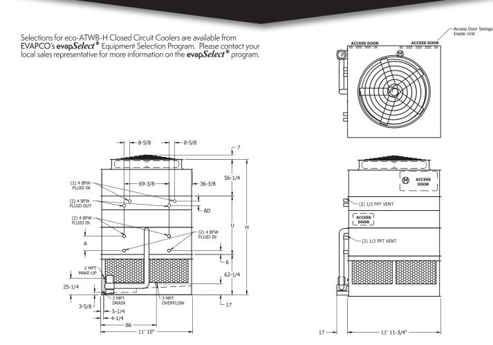
Note: The below table lists base unit dimensions and weights. See the table at the bottom Right of the Page for dry coil section dimensions and weight adds. Note: The number of coil connections doubles when the flow rate exceeds 900 GPM on eco-ATWB-H 12x12 models. This required option is referred to as the High Flow coil configuration.
