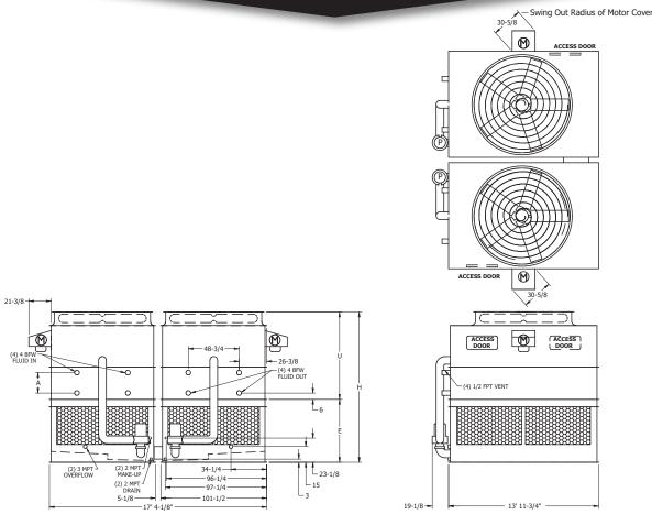
Note: The number of coil connections doubles when the flow rate exceeds 1,800 GPM on eco-ATW 17x14 models. This required option is referred to as the High Flow coil configuration.
