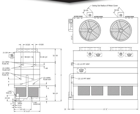
Note: The below table lists base unit dimensions and weights. See the table at the bottom Right of the Page for dry coil section dimensions and weight adds. Note: The number of coil connections doubles when the flow rate exceeds 900 GPM on eco-ATWB-H 9x21 models. This required option is referred to as the High Flow coil configuration.
