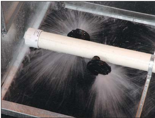
EvapJet™ nozzle compared to previous EVAPCO nozzles
