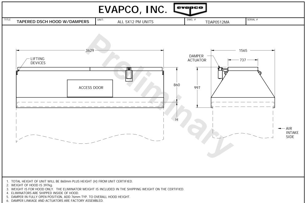
WIRING AND ACTUATOR CONTROLS FURNISHED BY OTHERS. 240 VOLT, 1 PHASE POWER SUPPLY REQUIRED.
